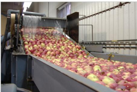
the rinse equipment indicates contamination but the source water is clean, you should clean out any nozzles, equipment and hoses with a sanitizer such as bleach.
